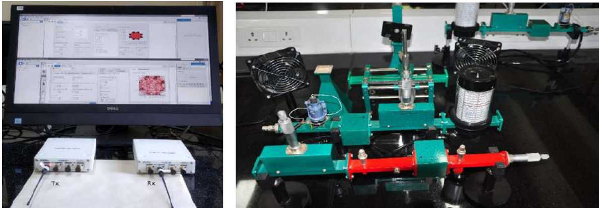
Communications and Microwave Lab, Left: Software Defined Radio (SDR) Kit, Right: Microwave Communication Set Up
