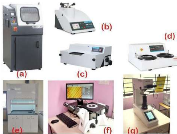
a) Abrasive cutting machine, b) Mounting press, c) Belt grinder, d) Polishing machine, e) Fume hood, f) Metallurgical microscope, g) Vickers hardness tester.
